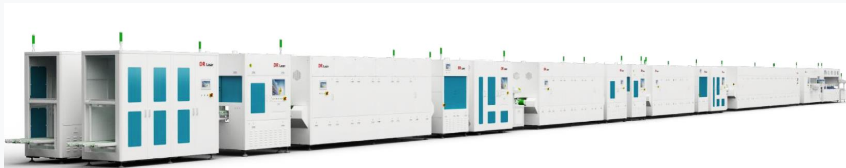
State-of-the-art Metallization Line for TOPCon and HJT including Pattern Transfer Printing
